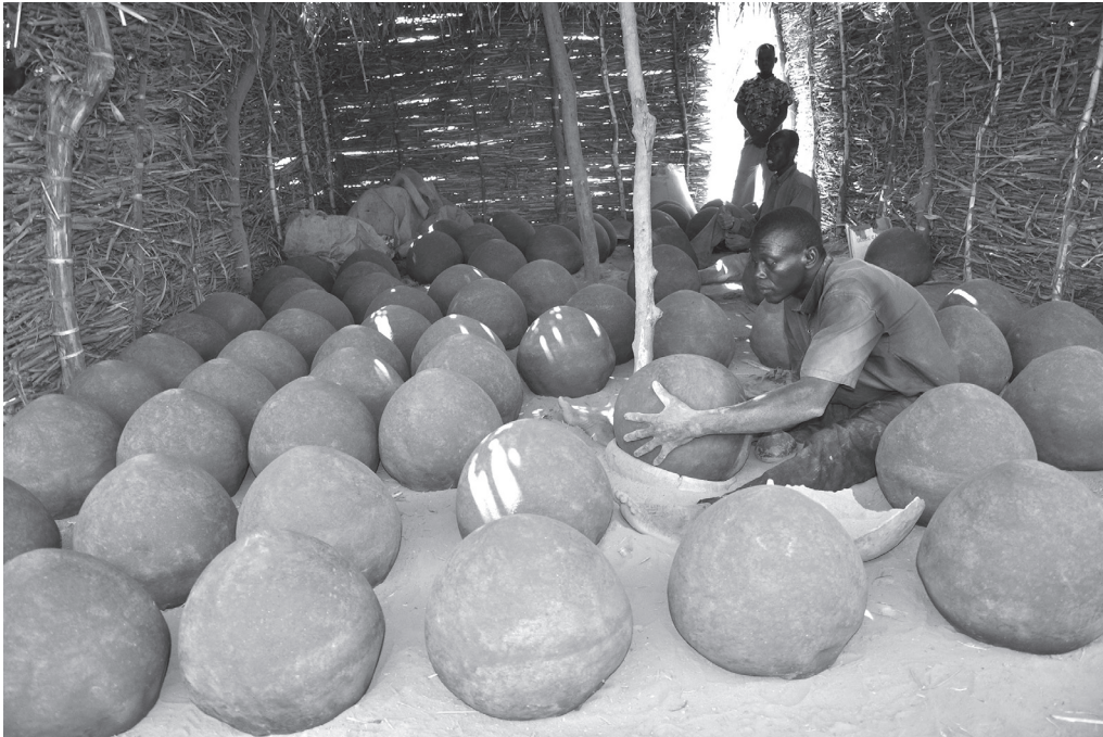
4 Interior of a workshop in the Dankawa district of Jiratawa. Vessels are shaped in three stages, in series of 20 to 60 (Photo ■■■)
