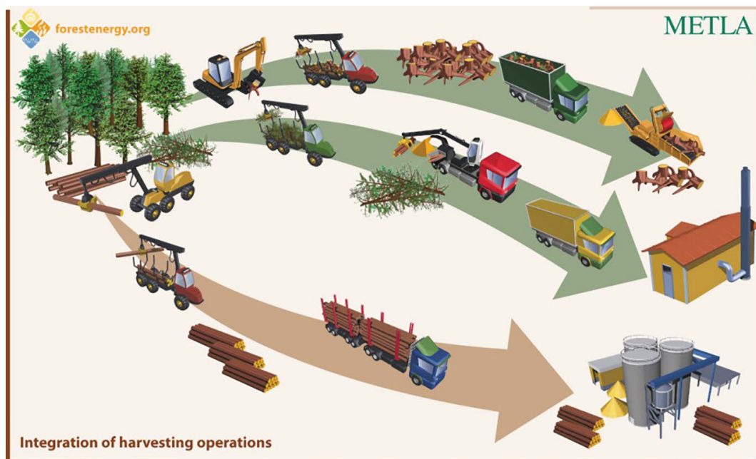
Figure 12. Supply chains for roundwood, logging residues and stumps from final fellings. Source: Forest Energy Portal.
