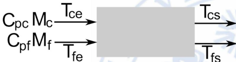
$$\frac{M_c C_{pc}}{M_f C_{pf}} = \frac{(T_{fs} - T_{fe})}{(T_{ce} - T_{cs})} \quad (260)$$
