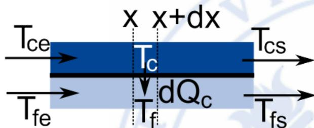
$$\frac{d(T_c - T_f)}{(T_c - T_f)} = -\frac{Ud\Omega}{M_c C_{pc}} \left[ \frac{(T_{ce} - T_{cs}) + (T_{fs} - T_{fe})}{(T_{ce} - T_{cs})} \right] \quad (272)$$
