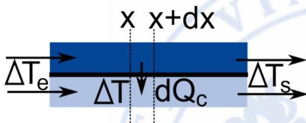
$$Q_C = U\Omega \frac{(\Delta T_s - \Delta T_e)}{\ln\left(\frac{\Delta T_s}{\Delta T_e}\right)} \quad (279)$$
