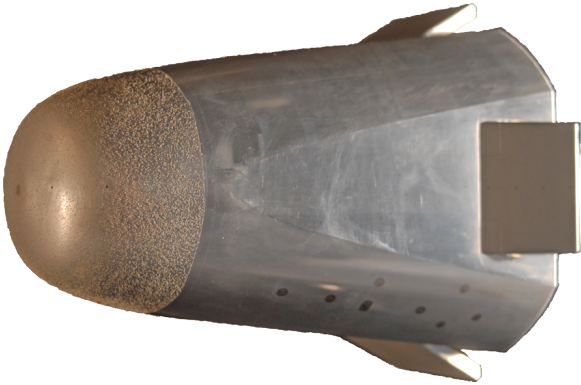
Figure 3. Model equipped with roughness \bar{k} = 0.194 mm and a density of 300 /cm 2
